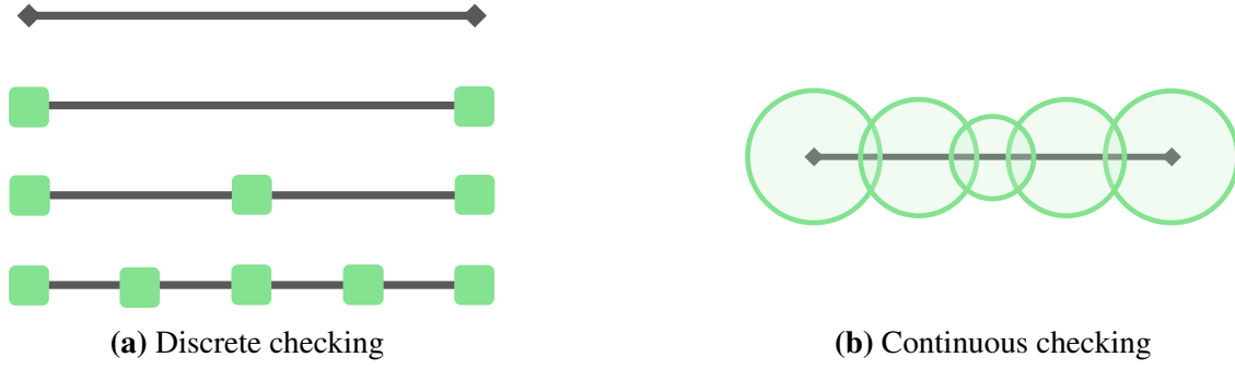
Figure 3.3: Illustration of discrete and continuous examination. Discrete examination verifies the middle point of the segments for better efficiency, where the green cubes indicate the examination points. When an edge is verified to be valid using discrete checking, it is still possible that a segment between two cubes is invalid, while the continuous checking in (b) does not have such a problem.
