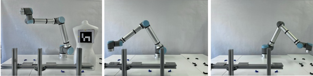
Figure 3.13: Robot experiment setup. The left figure shows a UR10e robot and a dynamic object with an ArUco marker attached for tracking purposes. Throughout the experiments, the robot travels between the two configurations of the middle and right figures.
