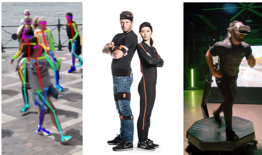
Figure 1.1.: Variety of recent motion capturing devices recording gait of individuals in public and private spaces from video or inertial measurement units (cf. OpenPose, VFXVoice, Virtuix).
