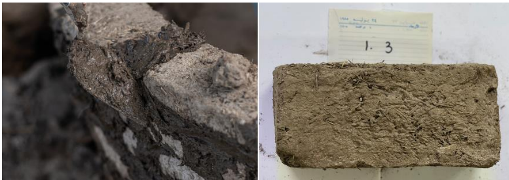
Figure 7. Wall construction process with mud mortar and mudbrick sample 1.3 in the laboratory in Cairo. Photos: Hussein Elsarnagawy (left), Nouran Mohamed (right)
