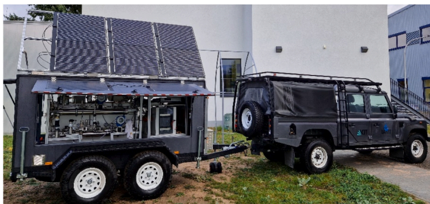
Fig. 1. Mobile lab equipped with the PV-membrane system (prototype VII) that is towed by a Land Rover Defender 130 for fieldwork in remote areas.
