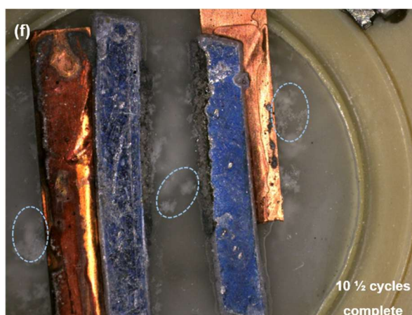
Figure 39: Overview of CuNa/CuNa symmetric cell with EC:PC 0.75 M NaPF 6 + 5% FEC electrolyte after 11 oxidations at 1.0 mA/ cm 2 .
