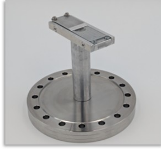
Figure 4.7.: Component that holds a glass slide. It includes a piece of aluminum that covers half of the glass slide. In principle other materials than glass can be mounted in this holder. The construction was made such that the holder can be mounted in any orientation without the possibility of dropping the glass slide. The holder is attached to a CF100 flange.
