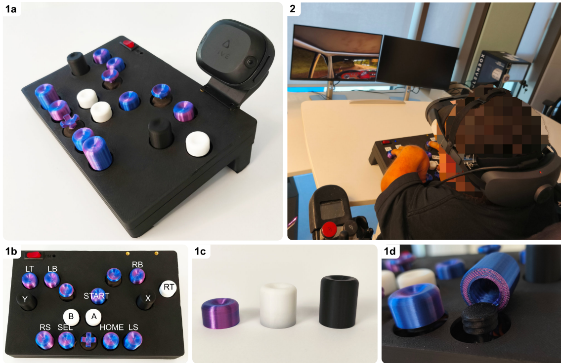
Fig. 8. Final iteration of Simon's case study. 1 The VR gamepad controller for Simon. a The controller has a static tilt and an interface for an HTC Vive Ultimate Tracker. b Controller layout with button mapping. c , d Height-adjustable buttons with screwing mechanism in different colors and sizes. 2 Simon playing Dirt Rally 2.0 with the final gamepad controller.
