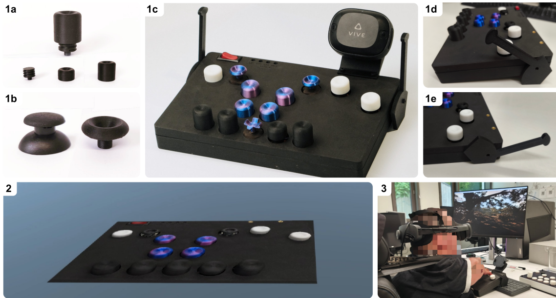
Fig. 7. Second iteration of Simon's case study. 1 VR gamepad controller with new features: a Height-adjustable buttons in two sizes with a screwing mechanism. b A comparison of old (left) and new (right) joystick caps. c VR gamepad controller with attached HTC Vive Ultimate Tracker. d, e Handles can change the controller tilt. 2 Virtual replica of the gamepad as seen in VR based on tracking data of the HTC Vive Ultimate Tracker. 3 Simon playing Resident Evil 7: Biohazard with the second iteration of the gamepad controller.
