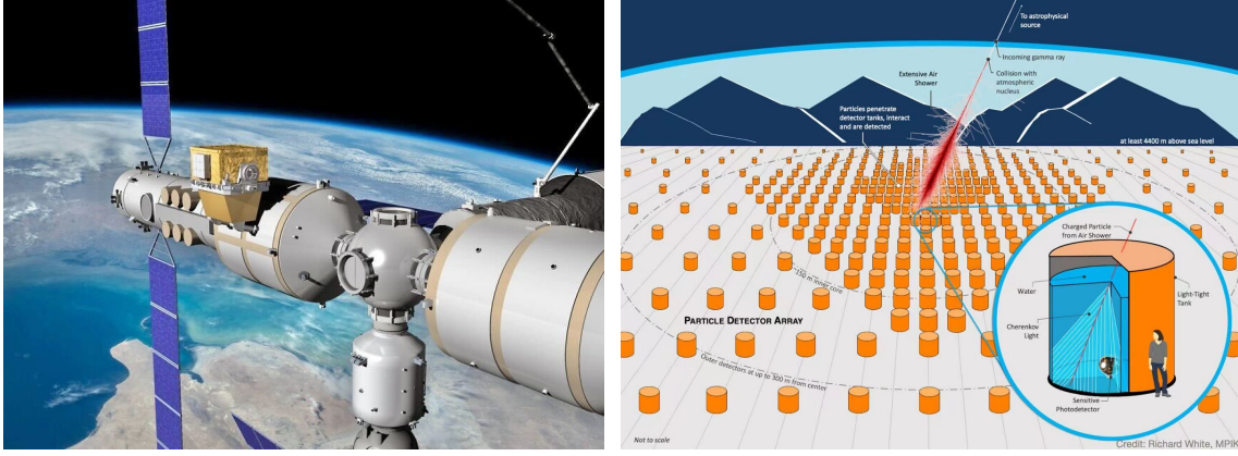
Figure 1.4: Left: Illustration of the HERD instrument, which will be installed on board the Chinese Space Station (CSS) around 2027, with a planned lifetime of 5–10 years (image taken from [86]). Right: Layout of the SWGO array with surface detectors arranged at a high-altitude site (4770 m) in Chile (credit: Richard White, MPIK).
