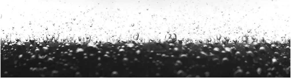
Figure 1.1: Boiling heat transfer on a heated rod in an annular gap. Experimental figure provided by Wefers et al. (2025a) obtained by using the COSMOS-L facility at KIT (refer to Wefers et al. (2025b) for details).
