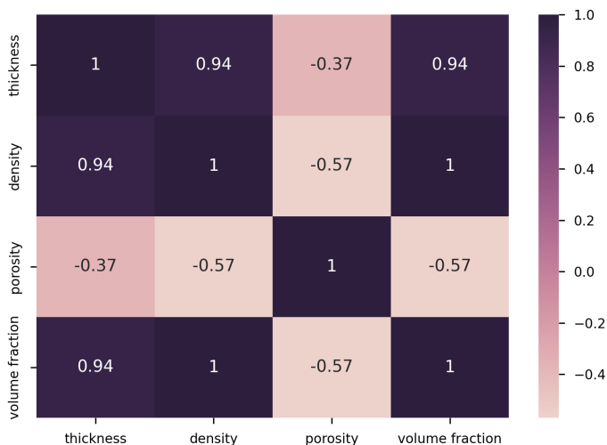
Figure 4.4: Heatmap showing the correlation between different target physical properties. The low variance and weak correlation of porosity with other properties explain the low R^2 score in predicting the porosity information of SEI configurations. Reproduced from [108] under the terms of the Creative Commons Attribution–NonCommercial–NoDerivatives (CC BY-NC-ND) license.
