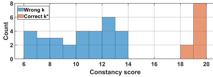
Figure 4.6.: SPFA score distribution: the correct key k^* yields a sharp, stable peak at the same \delta across pairs; wrong keys are near-uniform.
