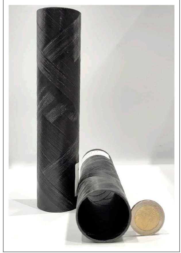
Figure 3. Wound preform of PA6 and carbon fibre.
