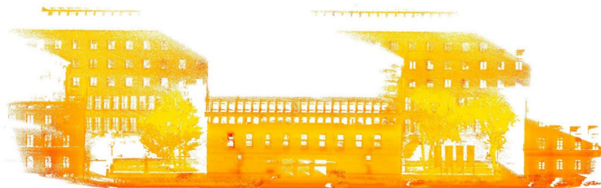
Fig. 10 Fused thermal point cloud of the test site
