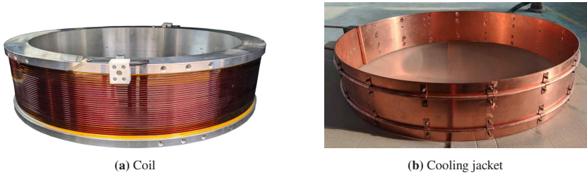
Figure 3.20: One of three external coils and cooling jacket for increased operation time.
