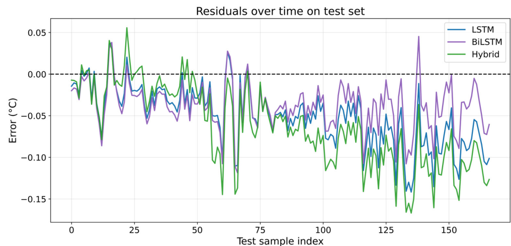
Figure 12. Time-resolved residual temperature errors for the LSTM, BiLSTM, and hybrid models, illustrating bounded and unbiased prediction behavior without drift.
