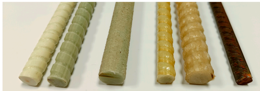
Figure 1. Overview of differently profiled rebars. From left to right: FRP-rebars with a milled helical groove, FRP-rebar with sand coating, FRP-rebars with a tight helical roving wrapping, conventional steel rebar.
