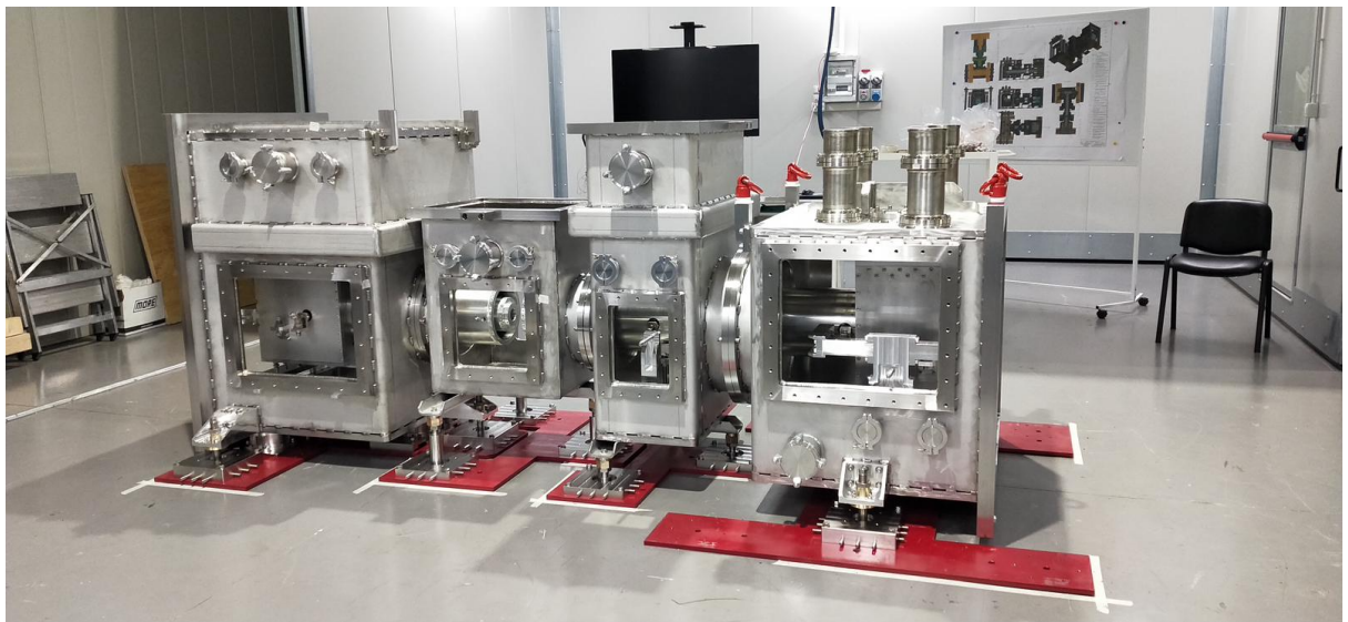
Figure 2.4: Mechanical assembly of a cryocooler-based cooling duct prototype developed at ARC (reproduced from [101], licensed under CC BY-NC-ND 4.0).
