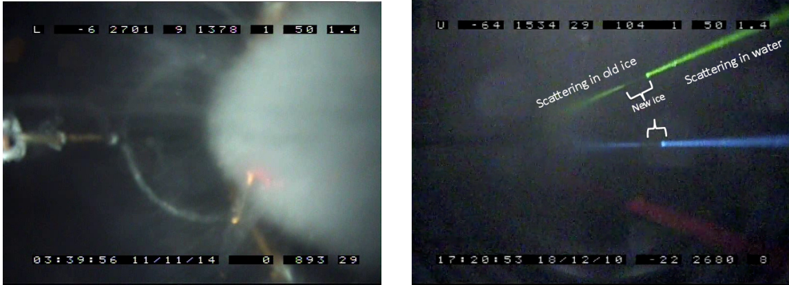
Figure 1: Images from integrated cameras shortly after deployment. Left: Upward-facing camera captures a milky, bubble-rich region on the right in contrast to the clear refrozen ice on the left. Right: Side-facing view shows significantly reduced scattering in the refrozen ice compared to the surrounding glacial ice.
