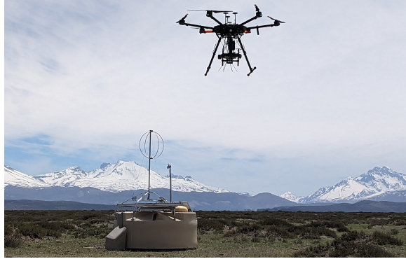
Figure 1: An upgraded surface detector station. The loop antennas on top are part of the Radio Detector. The image was taken during a calibration measurement with a reference radio source mounted on a drone.
