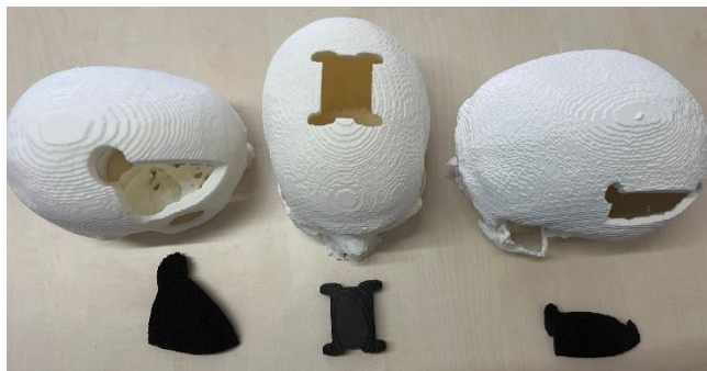
FIGURE 13. Bench-top view of “print-ready” implants generated by Version 3: Three skull phantoms with diverse defects are displayed alongside their black, 3-D-printed implants before seating. Each implant, produced directly from the network’s STL output, matches the defect geometry without requiring manual CAD edits or post-print sanding, an outcome consistent with version 3’s superior overlap and boundary metrics and unattainable with earlier Modified U-Net variants or other models
