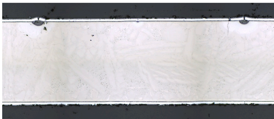
Fig. 12. Local failure positions of 25-μm sample after 1-hour oxidation at 1200 °C.
