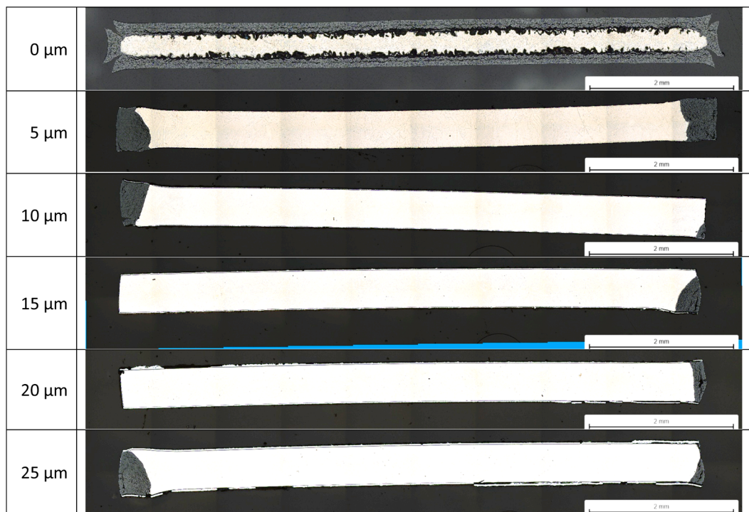
Fig. 6. Cross section micrographs of the samples after 2-hours oxidation at 1000 °C.
