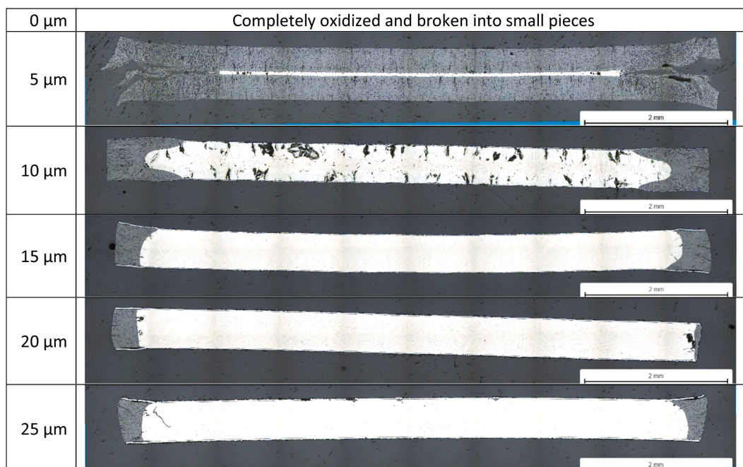
Fig. 10. Cross section micrographs of the samples after 1-hour oxidation at 1200 °C.
