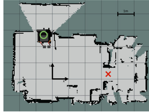
Fig. 2. Map of the experimental environment generated by RTAB-Map. The start and end positions are located in the upper left corner (green circle) and on the right side (red cross), respectively.
