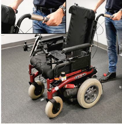
Fig. 1. Intelligent powered wheelchair being pushed by a human user, with force sensors mounted on the rear handles to measure input forces.
