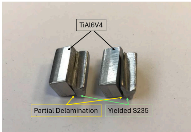
Fig. 10. Group A – Partial delamination and yielding after the shear strength test (sample #3).
