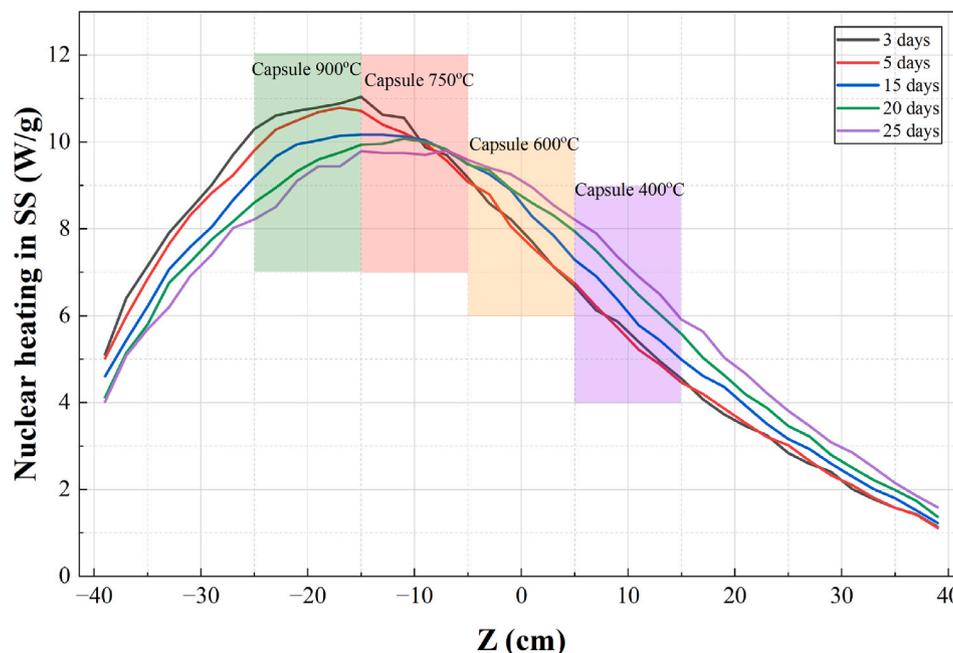
Fig. 1. Variation of the nuclear heating in SS during the irradiation cycle along the core length in B-180 channel.
