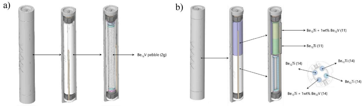
Fig. 4. Capsule design (a) at 750/900°C for pebbles. (b) 750/900°C for pellets/disks and cylinders.
