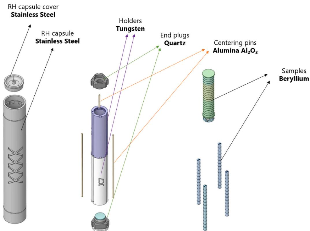
**Fig. 2.** Stainless steel BAMI RH capsule used for the irradiation of Be samples. The capsule has an outer diameter of 15 mm and is loaded in VIn element fuel element channel.
