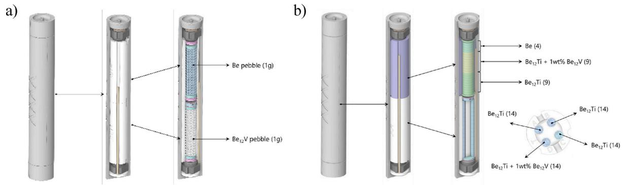
Fig. 3. Capsule design (a) at 400/600°C for pebbles. (b) 400/60000B0C for pellets/disks and cylinders.
