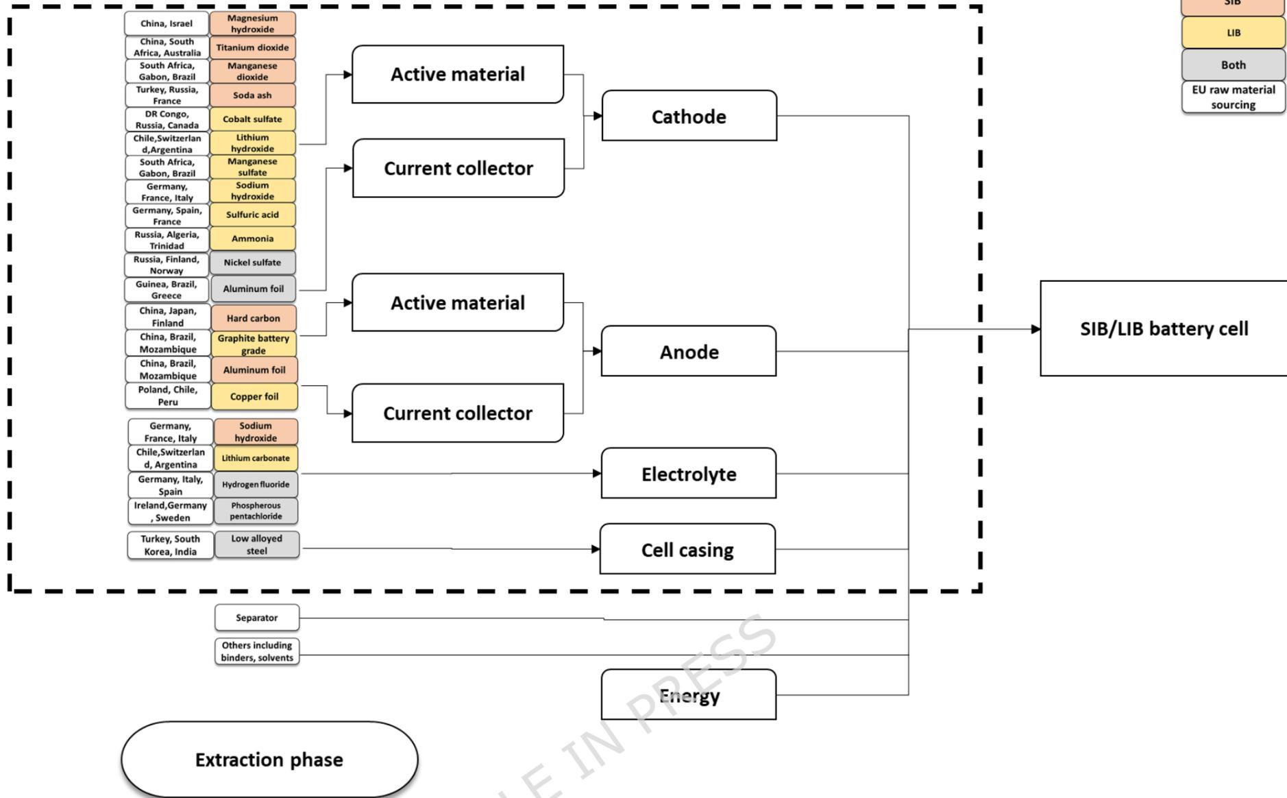
Figure 2: Product system and system boundary
