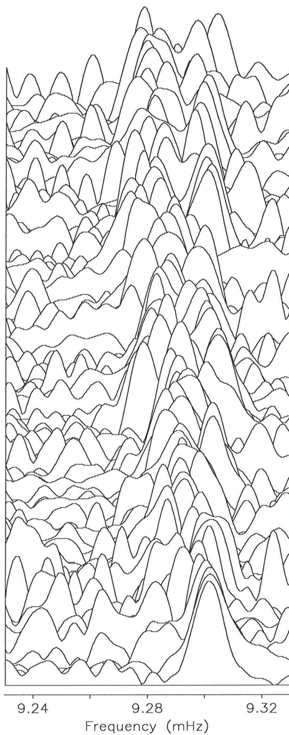
Figure 3.1 Perspective view of 86 vertical component amplitude spectra containing signal for the mode {}_{23}S_5 . The spectra are sorted according to the latitude of the recording station. Spectra recorded at the South Pole are in front and spectra from equatorial stations are in the back.
