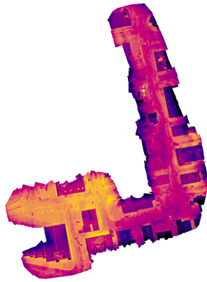
Figure A.5: Temperature drift in a case study set, with acquisition from top right to bottom left. Warm areas do not stem from underground heat (SWM).
