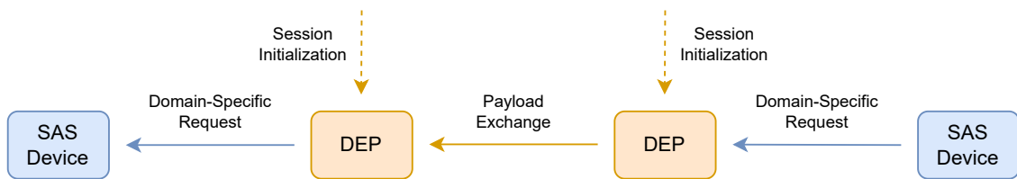
Fig. 12: Components and exchanged messages involved in a payload exchange between two SAS devices.
