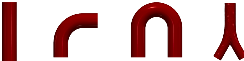
Fig. 10. Domains of interest (Dols) implemented in OpenLB for synthetic investigations regarding the parameter identification framework. From left to right: straight pipe, 90°-bended pipe, U-shaped pipe, bifurcation.
