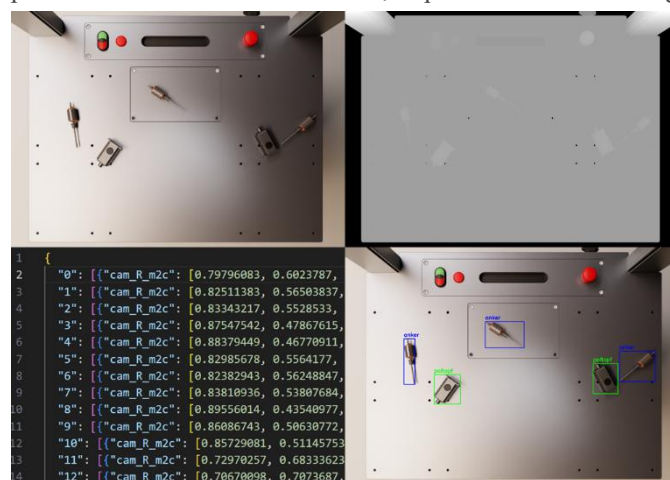
Fig. 1. Output from the simulation environment; Top left: Virtual RGB image, top right: Depth information in grayscale, bottom left: ground truth information, bottom right: visualization of the automatically labeled image with randomized object count, object position, lighting, and material properties.
