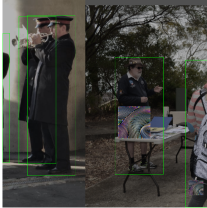
Figure 3.1: Example image as used during adversarial training after the augmentation pipeline. The ground truth bounding boxes are drawn in green. The added adversarial patches are located at the person in the center and on the bottom right below the backpack.
