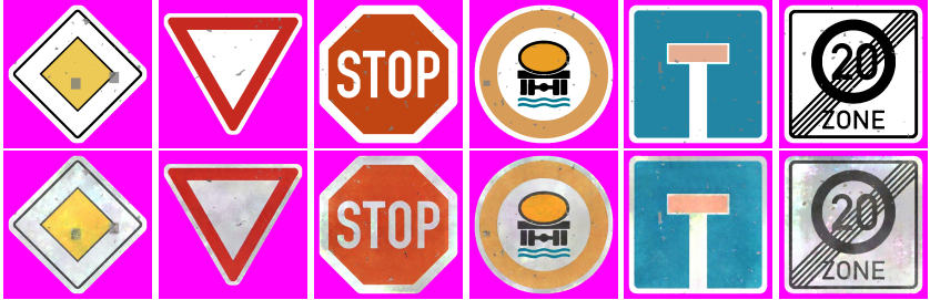
Figure 3.4: Results from the texture generation module used for generating SSG [32]. Upper row: procedurally generated template images; lower row: corresponding GAN interference results.
