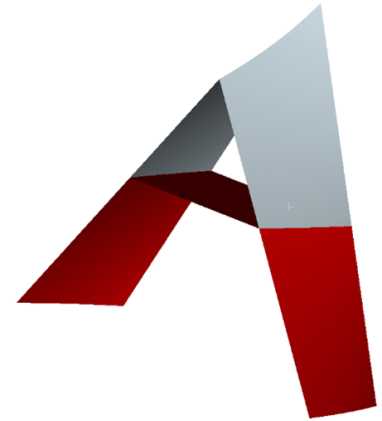
(b) Virtual substitute model of the tooth tip through profile extrapolation.
