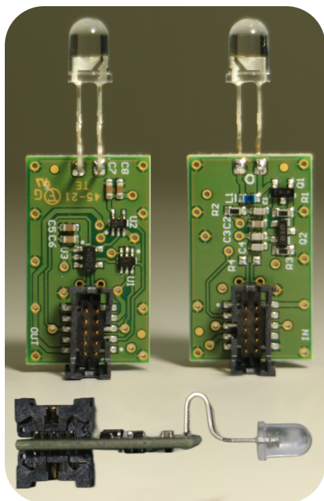
(a) Each flasher comprises a 25 mm by 15 mm PCB and a single outward pointing LED. Five of these LED elements wired in series via ribbon cables form a flasher daisy chain.
