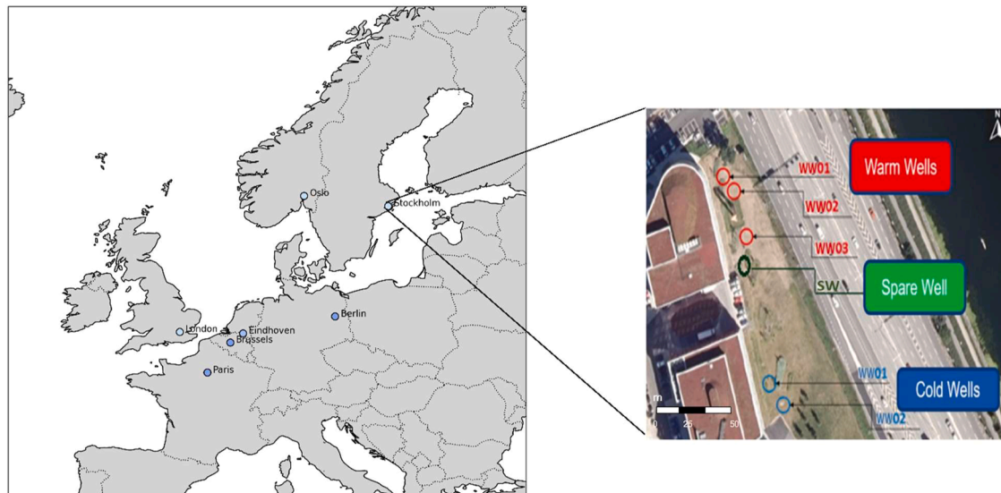
Fig. 8. ATES in Stockholm supplying heating to office buildings studied by Abuasbeh et al. (2021). The system includes a spare well, which was utilized to analyze the operational performance of the ATES system. (adapted and reproduced from (Abuasbeh et al., 2021), CC BY).
