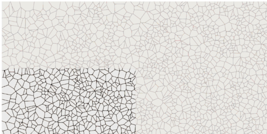
Fig. 6. Voronoi subset (black) used as porous domain in two-phase flow simulation. The porous area simulated in the monophasic scenario shown in light grey.
