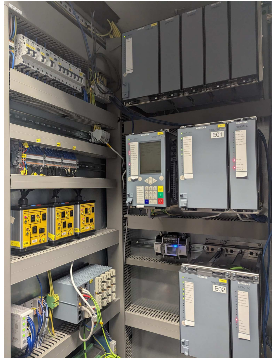
(b) Physical setup of I/O Boxes and Switchgear Simulators (yellow boxes) among other equipment in the lab.
