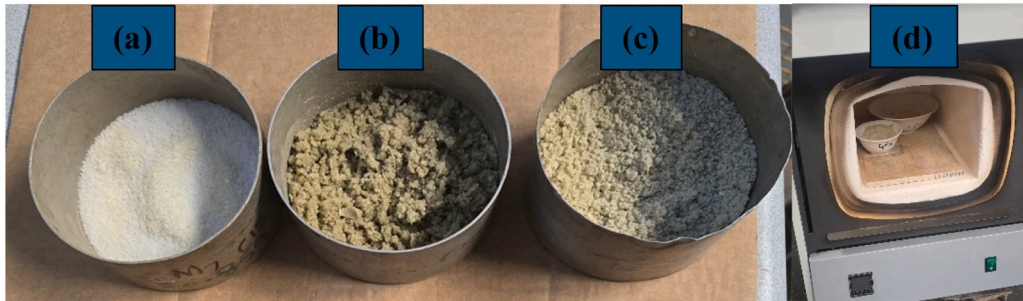
Fig. 2. Visual appearance of WGP-sodium hydroxide mixtures: (a) E1, (b) E4, (c) E7 before and (d) during thermal activation in muffle furnace.
