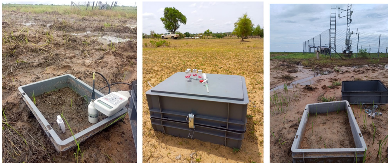
Fig. 2. Chamber-based greenhouse gas sampling plots; closed (middle) and opened for soil moisture and soil temperature measurements (left and right) in a rice field at Janga, Upper-East Ghana.
