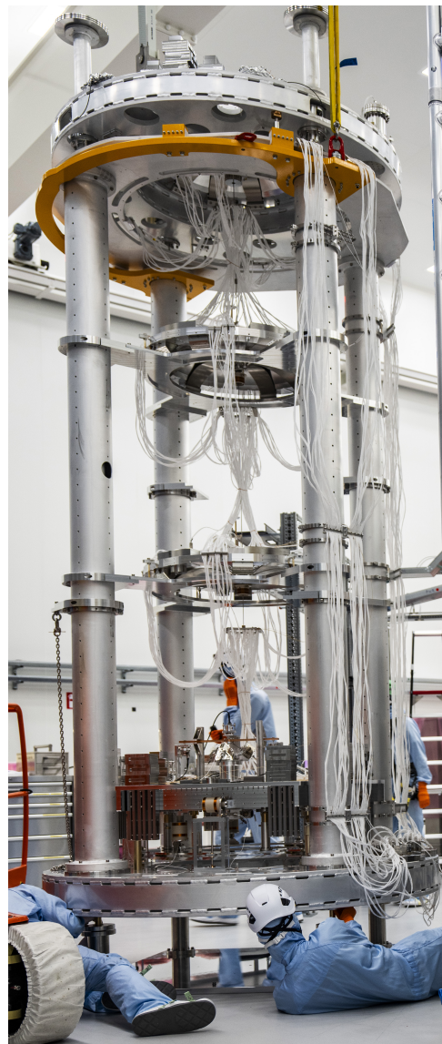
Figure 2: Picture of the constructed BST suspension of ETpathfinder located in the cleanroom outside the vacuum system.
