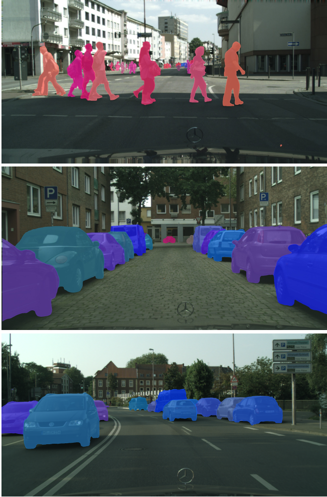
Figure 4.7: Sample instance segmentation results from the Cityscapes dataset using the Dirichlet MLE + ILVI model with the EfficientNet backbone. The visualization presents color-coded masks for pedestrians and vehicles across diverse urban scenes, demonstrating the model’s segmentation performance. Different colors distinguish object instances, showcasing the model’s ability to identify and separate individual objects within complex environments.
