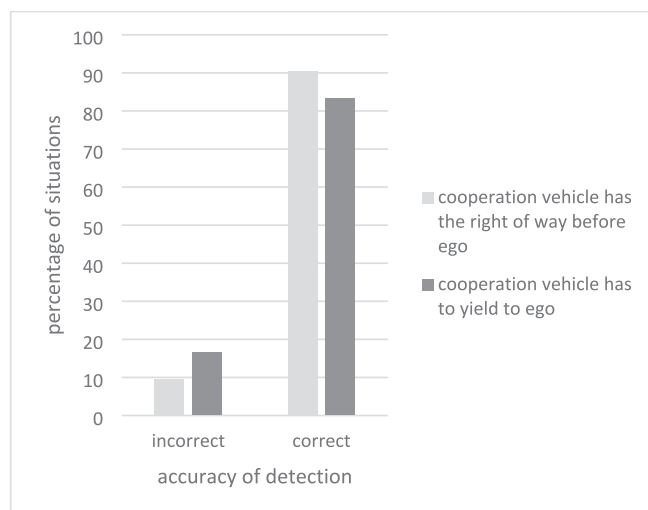
Fig. 3. Percentage of correctly and incorrectly identified directions of travel of the cooperation vehicle, depending on its right-of-way relative to the ego vehicle.
