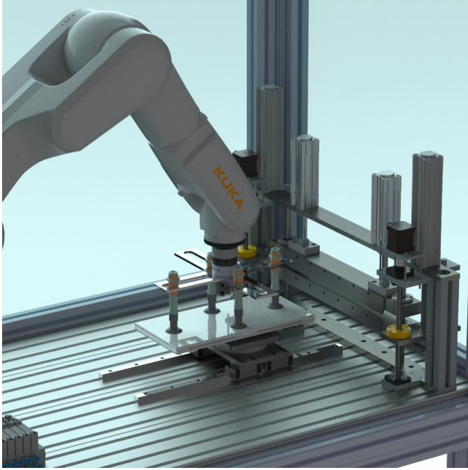
Fig. 8. Final design of the disassembly station with guillotine cutting mechanism.
