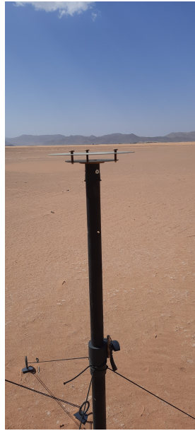
Figure 4.23.: Flat-plate sampler (FPS) used in the J-WADI campaign, adapted from Ott and Peters (2008). Positioned 10m from the rotating mast, it consists of two brass plates at a distance of 16mm and a circular substrate (diameter = 25 mm) in the center of the bottom plate. Figure by TT- Prof. Dr. M. Klose.
