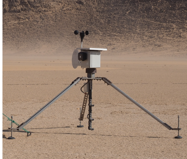
Figure 4.3.: SANTRI instrument to measure saltation and retrieve flux density to obtain threshold friction velocity.
