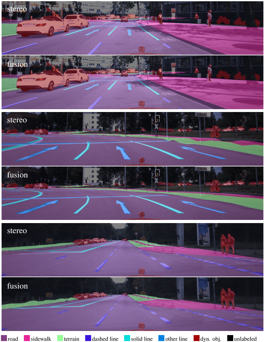
Figure 5.11: Qualitative evaluation of the dense surface feature map M_{DS} in three scenarios, comparing different reconstruction approaches. In each pair, the top image shows the stereo-based result, and the bottom image shows the fusion-based result. Areas in red are identified as occluded by dynamic objects, further described in Section 7.2.1. While both methods produce comparable reconstructions in the central region, the fusion-based approach provides greater accuracy near the boundaries of the field of view.
