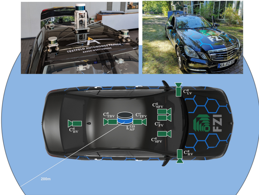
Figure 4.1: Research Vehicle BerthaOne [TSP18] with corresponding sensor suite. The specifications of each sensor are further listed in Table 4.1.
