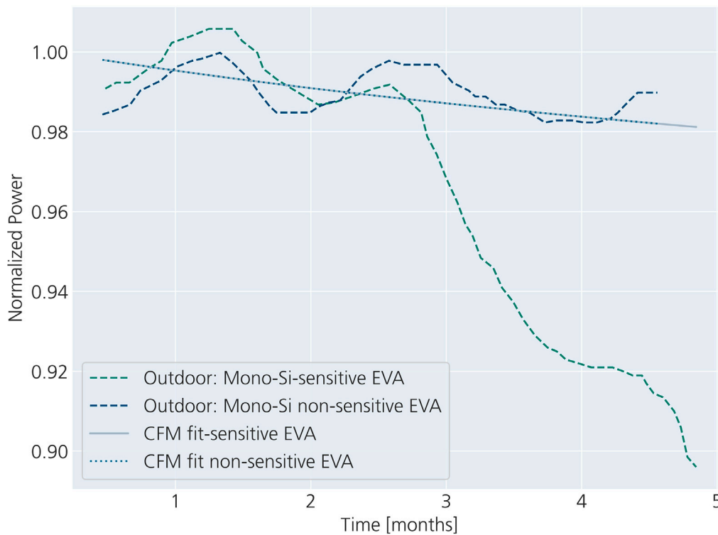
Fig. 7. Comparison of CFM's prediction against PID outdoor data from Berghold et al. (2013).
