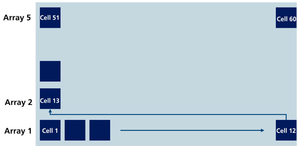
Fig. 2. A typical arrangement of a 60 cell module with 5 substrings inside MAPLE. Cells 1, 12, 51 and 60 are corner cells. Cells 2-12, 13, 25, 26, 38, 39, 50 and 52-59 are side cells.
