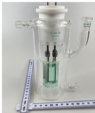
FIGURE 2 | Activation of nickel foam electrodes in aq. NiSO 4 and NaOH. The NiOOH layer is easily distinguished from unfunctionalized foam by its dark appearance.
