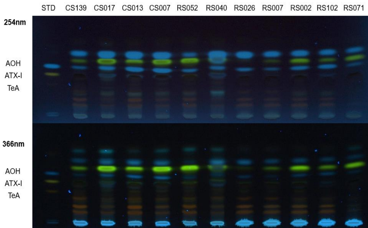
Figure 30: TLC of the first half of the A. alternata strains from Peru and Chile after 10 days of incubation at 28 °C in darkness on YES Medium. Along with the toxin extracts, a Standard mix was applied to the TLC plate containing AOH, ATX-I, and TeA. The same TLC plate is shown with irradiation of UV light at 254 nm and 366 nm. The mobile phase consists of toluol /ethyl acetate/formic acid (60:35:5, v/v/v).
