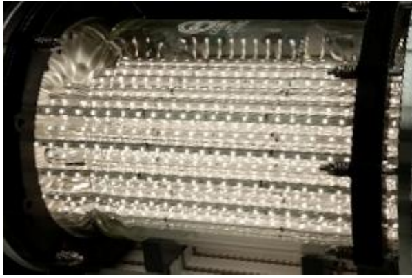
Figure 64: Empty cptPBR containing 37 light bars, with 72 LED spots per bar.
