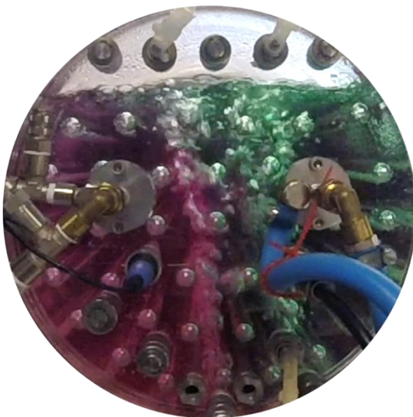
Figure 28: Photograph of the cptPBR cross-section using the gassing geometry 2×T14p1 in red cabbage coloring experiments after base injection.
