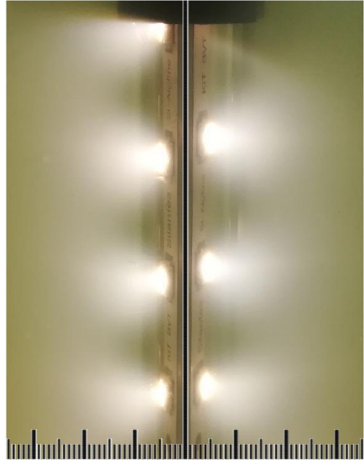
Figure 74: Photograph of LED spots of one light bar in a glass tube from the cptPBR in microalgal suspension ( cx = 26.5 \text{ g}\cdot\text{m}^{-3} ) with approximate cm/mm scale.
