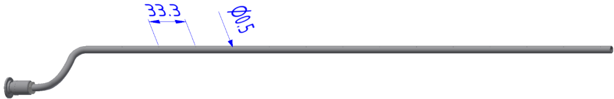
Figure 20: Engineering drawing of the gassing tube (15 pores, \text{Ø} 0.5 \text{ mm} ) initially installed in the cptPBR. This tube (T15p0.5) served as the experimental reference case.
