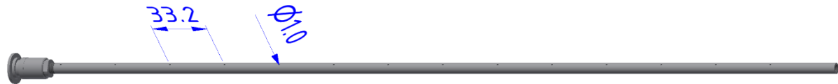
Figure 21: Engineering drawing of the gassing tube T14p1 with 14 pores ( \text{Ø} 1.0 \text{ mm} ). The tube was used for experimental testing.
