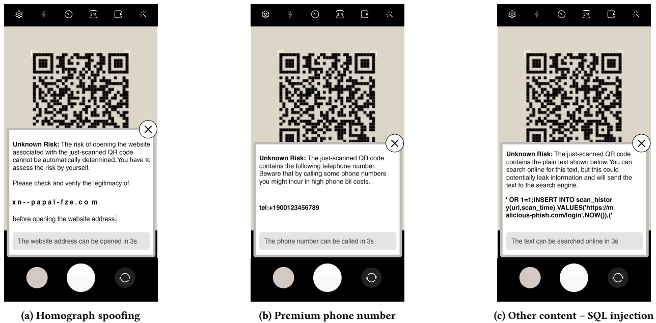
Figure 20: Examples of SEQ2 1.0’s warnings for: homograph spoofing (a), premium phone number (b), and an SQL injection (c).
