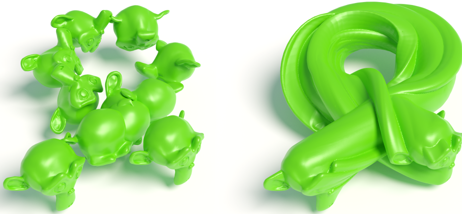
Figure 8.8: Swept volume of a sample object along a self-intersecting trajectory.
